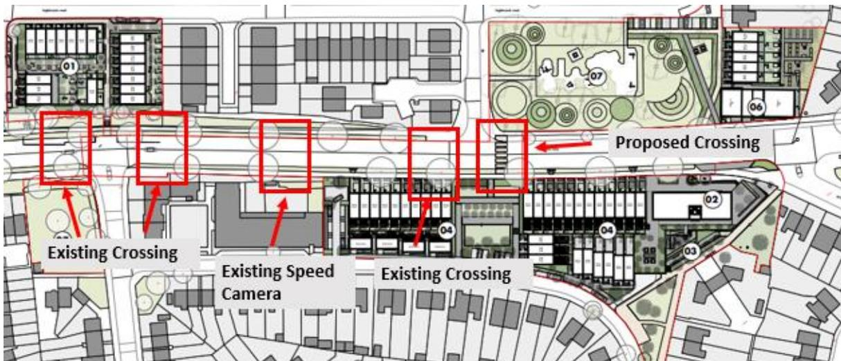
**Figure 1 Existing and proposed crossing on Rochester Way**
